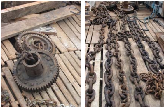
Figure 10. Scrap metal and chains used as ground tackle for the moorings (onboard MV 'Duta Daerah').
