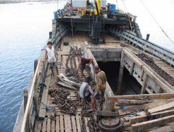
Figure 8. Ground tackle being prepared for deployment onboard the MV 'Duta Daerah'.
