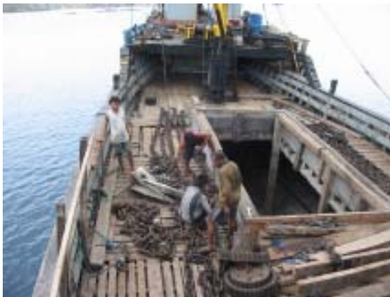
Figure 8. Ground tackle being prepared for deployment onboard the MV 'Duta Daerah'.
