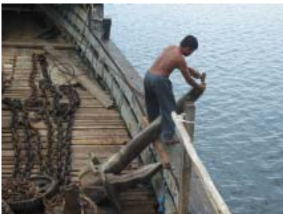
Figure 9. One of the two anchors for a 'Big Boat' being prepared for deployment onboard the MV Duta Daerah.
